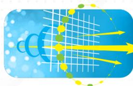
This provides 30% improved performance over conventional units since it reflects light onto the landing spot thereby stimulating the natural landing behaviour of flying insects.
